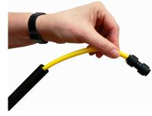
Pull out the gooseneck from the top of the pole and disconnect the pole hose from the John Guest connector under the gooseneck (see photo). Then pull the hose out of the pole.
