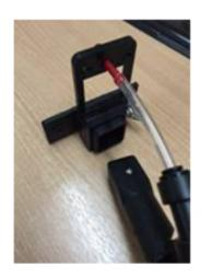
Fit the Mount around the brush socket or Vikan adapter and tighten the nut. Connect the Quick-Loq Angle Adapter and connect the hose that feeds through the Angle Adapter to the black Push-Fit Straight Connector.
